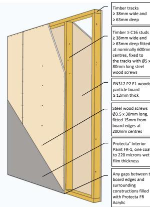
≥ 63mm deep fitted at nominally 600mm the tracks with Ø5 x EN312 P2 E1 wooden Steel wood screws Ø3.5 x 30mm long, Paint FR-1, one coat
